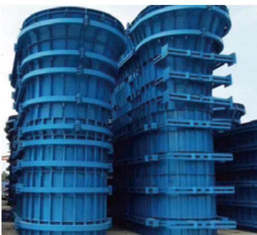
Steel Formwork for Pier 墩柱钢模板
